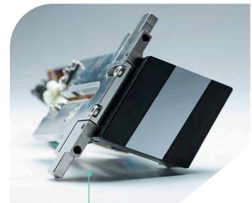
Samba printhead. Not visible to the naked eye, 2048 nozzles are contained in the silver-coloured silicon chip which measures just 44 mm wide by 18 mm deep.
